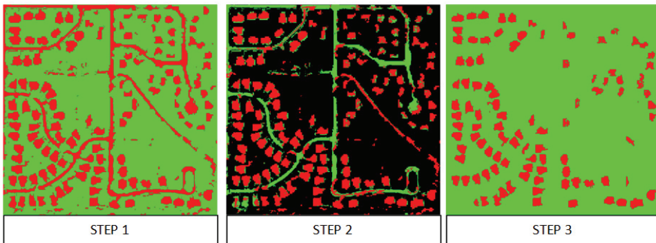
Fig. 6. Illustration of the outcomes produced by the evolutionary framework for each step considered. Step 1 outputs a binary image containing asphalt-based material and background. Step 2 uses the results of step 1 to generate another image discriminating asphalt rooftop from other asphalt-based material. Step 3 uses the output from step 2 containing group of connected pixels and filter them based on geometric properties.
